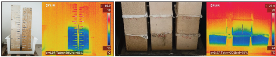
Figure 1: example of visible imaging and thermography of pietra leccese and carparo for mono-block and carparo , pietra leccese and tuff for multi-blocks.
